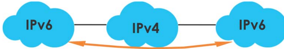
Figure 264 IPv6 over IPv4 Network
