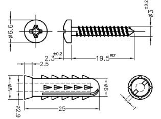
Figure 6 GS1100-16/GS1100-24E screw specs
