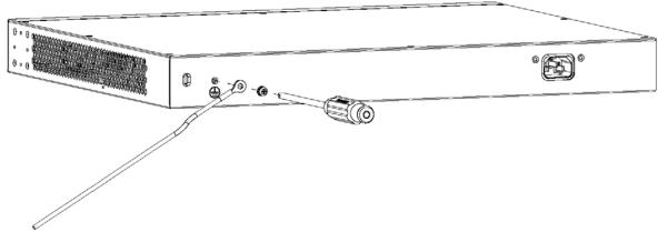
3 Attach the other end of the ground cable to a grounding bar located on the rack where you install the Switch or to an on-site grounding terminal.
