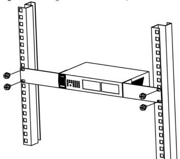
Figure 9 Mounting the Switch on a Rack (GS1100-16 and GS1100-24E)
