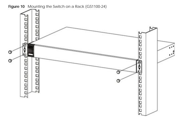
2 Using a #2 Philips screwdriver, install the M5 flat head screws through the mounting bracket holes into the rack.
