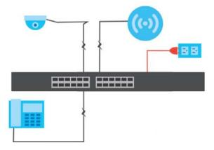
PoE ports support both the IEEE 802.3af Power over Ethernet and IEEE 802.3at High Power over Ethernet standards.
