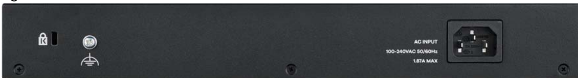
Figure 50 Rear Panel: GS1900-24 A1
