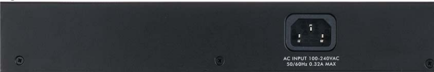
Figure 49 Rear Panel: GS1900-24E B1
