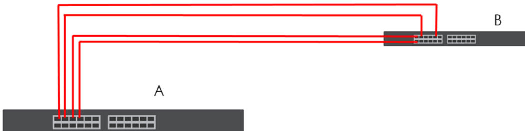
Figure 112 Trunking Example – Physical Connections
