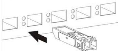
Figure 67 Connecting the Fiber Optic Cables
