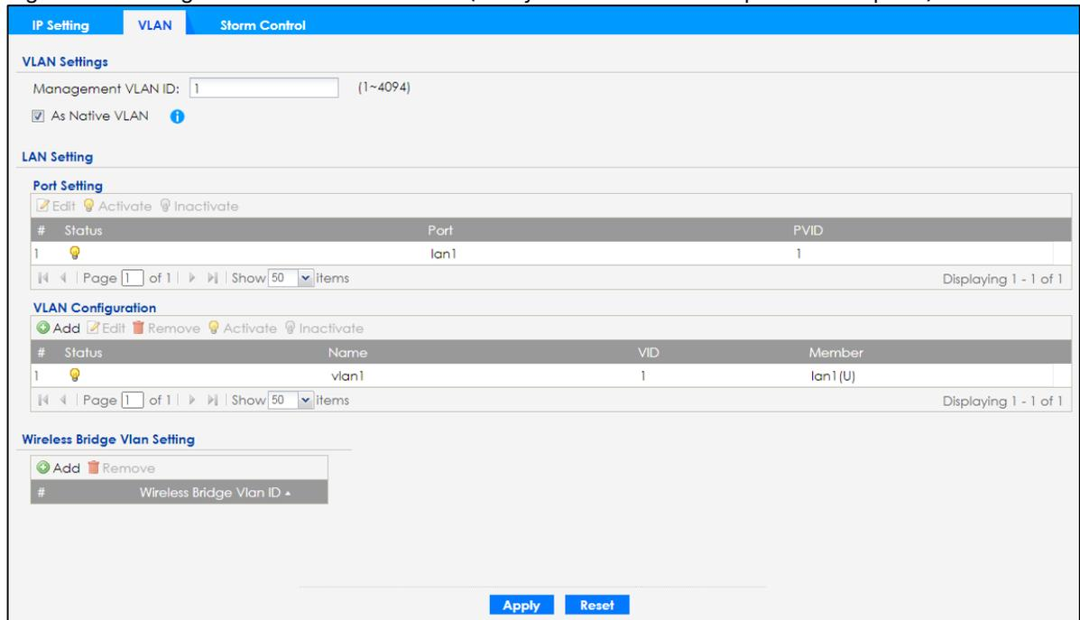
Figure 117 Configuration &gt; Network &gt; VLAN (for Zyxel Device with one Ethernet port)
