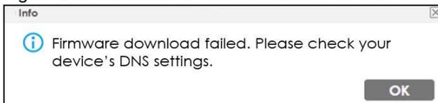
Firmware download failed. Download the new firmware manually from the Zyxel website. Then, go to the Maintenance > File Manager > Firmware Package screen to upload the new firmware.
