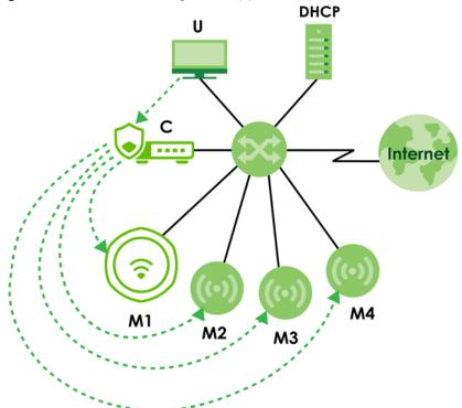
Figure 173 Controller Managed AP Application
