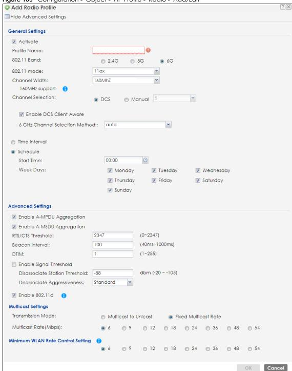
Figure 105 Configuration > Object > AP Profile > Radio > Add/Edit
