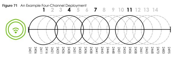
However, some regions require the use of other channels and often use a safety scheme with the following four channels: 1, 4, 7 and 11. While they are situated sufficiently close to both each other and the three so-called "safe" channels (1,6 and 11) that interference becomes inevitable, the severity of it is dependent upon other factors: proximity to the affected AP, signal strength, activity, and so on.
