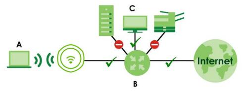
MAC addresses that are not listed in the layer-2 isolation table are blocked from communicating with the Zyxel Device's WiFi clients except for broadcast packets. Layer-2 isolation does not check the traffic between WiFi clients that are associated with the same AP. Intra-BSS traffic allows WiFi clients associated with the same AP to communicate with each other.
