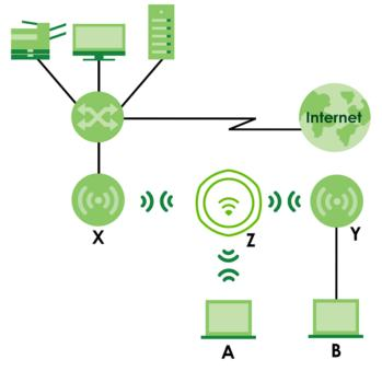
When the Zyxel Device is in **Repeater** mode, repeater security between the Zyxel Device and other repeater is independent of the security between the WiFi clients and the AP or repeater. When repeater security is enabled, both APs and repeaters must use the same pre-shared key. See Section 11.2 on page 112 and Section 14.2 on page 167 for more details.
