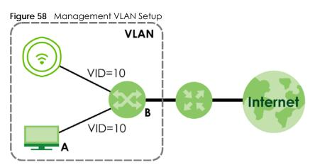
In the figure above, to access and manage the Zyxel Device from computer **A**, the Zyxel Device and switch **B**'s ports to which computer **A** and the Zyxel Device are connected should be in the same VLAN.
