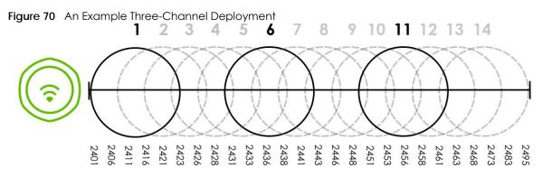
Three channels are situated in such a way as to create almost no interference with one another if used exclusively: 1, 6 and 11. When an AP broadcasts on any of these 3 channels, it should not interfere with neighboring APs as long as they are also limited to same trio.
