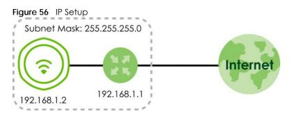
The figure above illustrates one possible setup of your Zyxel Device. The gateway IP address is 192.168.1.1 and the managed IP address of the Zyxel Device is 192.168.1.2 (default), but if the Zyxel Device is assigned an IP address by a DHCP server, the default (192.168.1.2) will not be used. The gateway and the Zyxel Device must belong in the same IP subnet to be able to communicate with each other.
