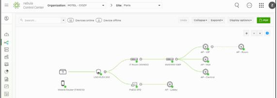
Note: Make sure your network firewall allows TCP ports 443, 4335, and 6667 as well as UDP port 123 so the Zyxel Device can connect to and sync with the NCC.
