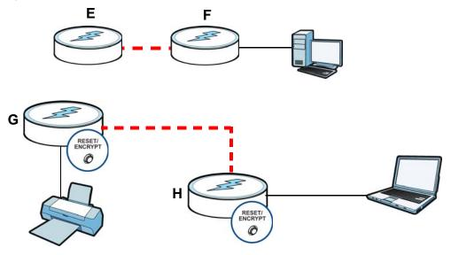
If the HomePlug ( ) lights on both powerline devices do not light up, the powerline devices are not connected. Repeat the connection process, making certain you press the **RESET/ENCRYPT** buttons for the correct time and within two minutes of each other. If that does not work see Section 6.4 on page 48 for suggestions.
