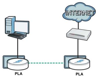
Connect your PLA to an Internet gateway such as a modem and plug it into an ordinary power outlet in your home. Plug a second PLA into another power outlet and connect a computer to the PLA for Internet access. Your network can be further expanded by plugging additional PLAs into other outlets in your home and connecting other computers or network devices (for example, a printer) to them.
