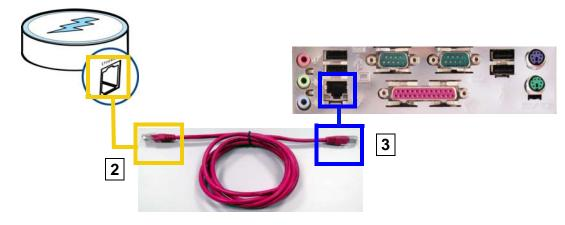
Figure 21 Connect Your Powerline Adapter to a Computer
