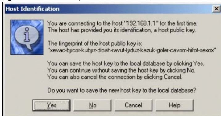
Figure 682 SSH Example 1: Store Host Key
