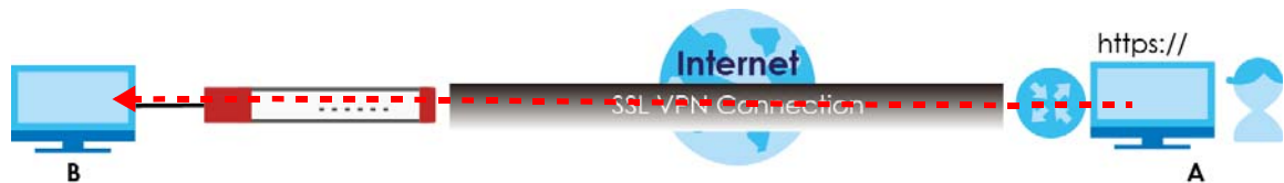
Figure 638 SSL-protected Remote Management
