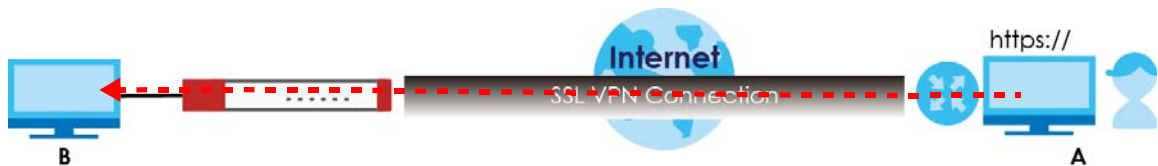
Figure 636 SSL-protected Remote Management
