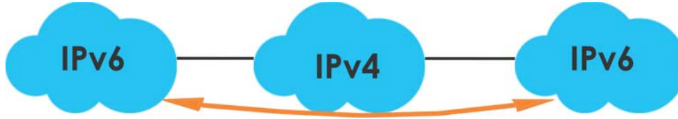
Figure 258 IPv6 over IPv4 Network
