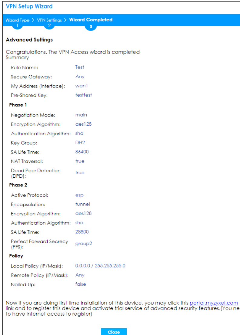
Figure 101 VPN for Configuration Provisioning Advanced Wizard: Finish
