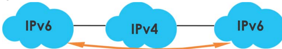
Figure 208 IPv6 over IPv4 Network
