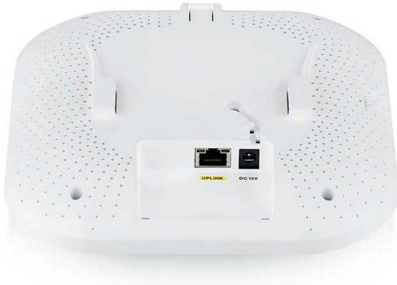
Figure 23 WAX640S-6E, WBE660S Ports
