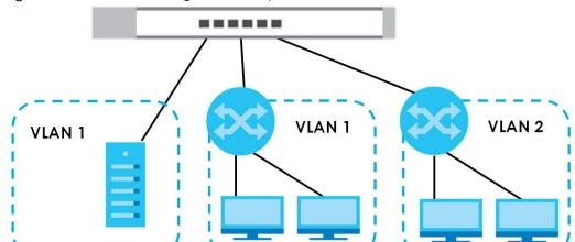
Figure 5 Shared Server Using VLAN Example
