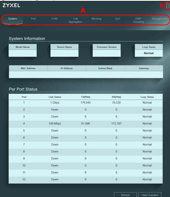
Figure 22 Web Configurator Layout
