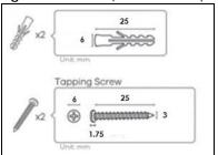
Figure 9 Screw Specifications (XGS1250-12)
