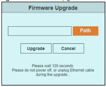
Type the path and file name of the firmware file you wish to upload to the Switch in the text box or click **Path** to locate it. After you select the firmware file, click the **Upgrade** button to load the new firmware.
