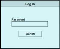
4 The following screen displays if you log into the Switch for the first time. Enter a new password using the keyboard characters ("a – z", "A – Z", "0 – 9", ~!@#\$%^&\*()\_+`-={}[]::<>./\). The password must be 8 to 15 characters long. Retype it to confirm and click **Apply** to view the first Web Configurator screen.
