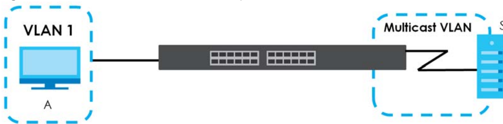
Figure 239 MVR Multicast Television Example
