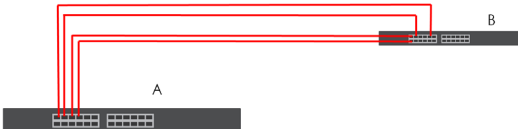
Figure 176 Trunking Example – Physical Connections
