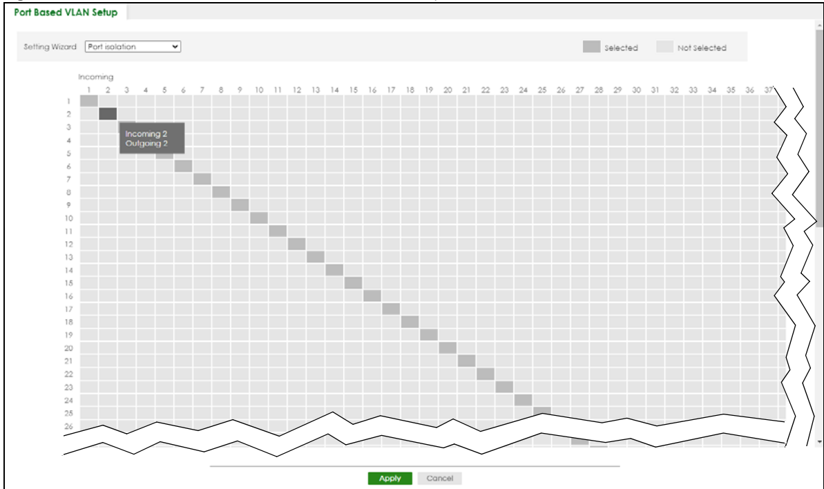
Figure 349 SWITCHING &gt; VLAN: Port Based VLAN Setup (Port Isolation)
