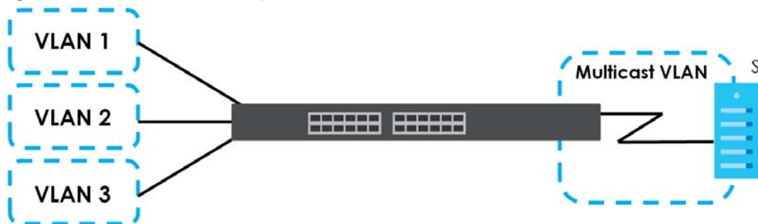
Figure 238 MVR Network Example
