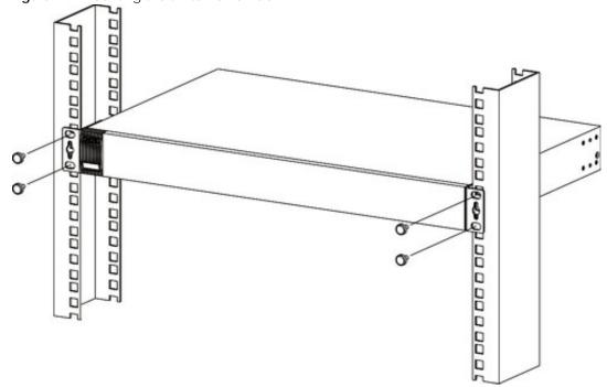
2 Using a #2 Philips screwdriver, install the M5 flat head screws through the mounting bracket holes into
