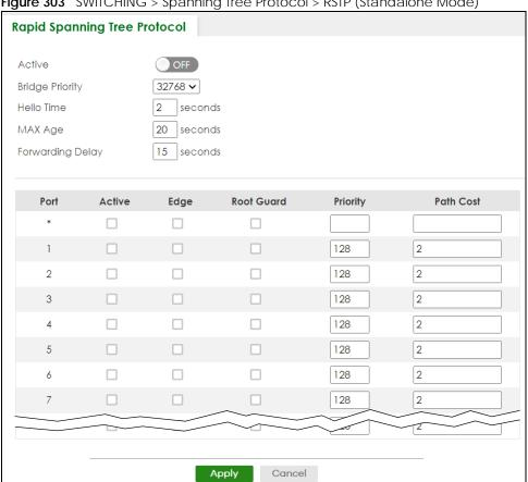
Figure 303 SWITCHING > Spanning Tree Protocol > RSTP (Standalone Mode)
