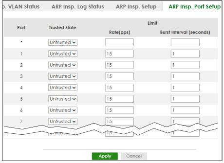
Figure 454 SECURITY > IPv4 Source Guard > ARP Inspection > ARP Insp. Port Setup (Stacking Mode)
