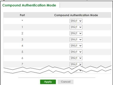
Figure 481 SECURITY > Port Authentication > Compound Authentication Mode (Stacking Mode)
