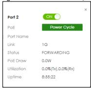
The port details pane includes the **Power Cycle** button for PoE models (turn the power off and then back on again), displays information such as link speed, status, PoE draw (for PoE models), port utilization, up time and has an ON/OFF switch button. Click the switch button to enable/disable the port.
