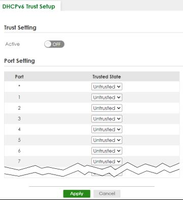
Figure 469 SECURITY > IPv6 Source Guard > DHCPv6 Trust Setup (Stacking Mode)
