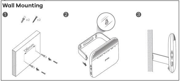
Note: Wall-mount the Zyxel Devices vertically. Attach the bracket to your Zyxel Device with the bracket holes facing down.
