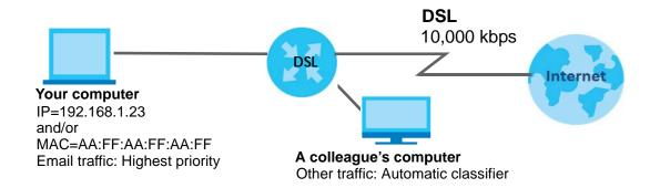
Click Network Setting > QoS > General and click the QoS button to enable. When the switch goes to the right ( ), the function is enabled. Set your WAN Managed Upstream Bandwidth to 10,000 kbps (or leave this blank to have the Zyxel Device automatically determine this figure). Click Apply.
