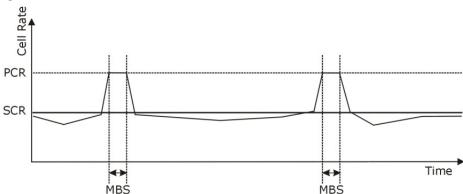
Figure 86 Example of Traffic Shaping
