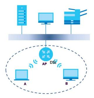
The wireless network is the part in the blue circle. In this wireless network, devices **A** and **B** use the access point (**AP**) to interact with the other devices (such as the printer) or with the Internet. Your Zyxel Device is the AP.
