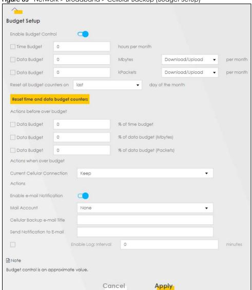
Figure 83 Network > Broadband > Cellular Backup (Budget Setup)
