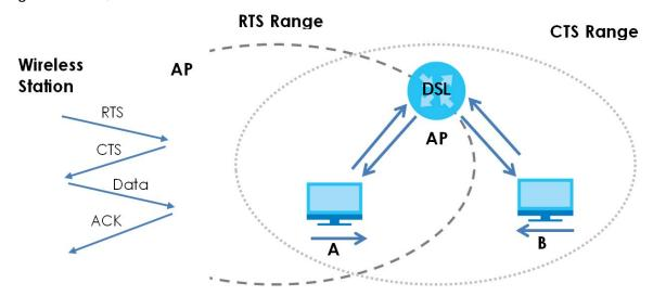
When station **A** sends data to the AP, it might not know that the station **B** is already using the channel. If these two stations send data at the same time, collisions may occur when both sets of data arrive at the AP at the same time, resulting in a loss of messages for both stations.
