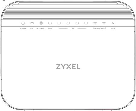
Figure 13 VMG3625-T50A Front Panel
