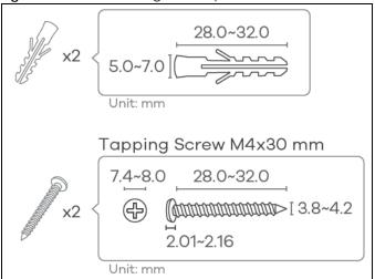
3 Use the holes on the bottom of the Zyxel Device to hang the Zyxel Device on the screws.
