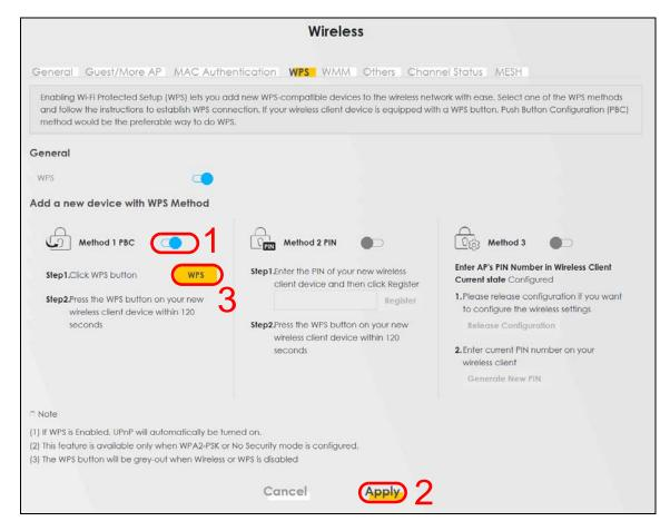
Note: Your Zyxel Device has a WPS button located on its side panel as well as a WPS button in its configuration utility. Both buttons have exactly the same function: you can use one or the other.
