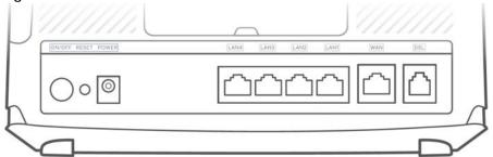
Figure 28 VMG3925-B10B Rear Panel
