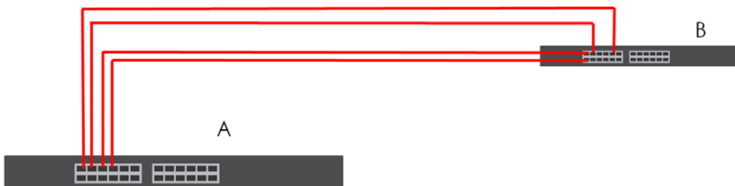
Figure 123 Trunking Example – Physical Connections
