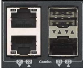
Figure 20 Combo Port Example: 10 Gigabit Port and SFP+ Transceiver Slot
